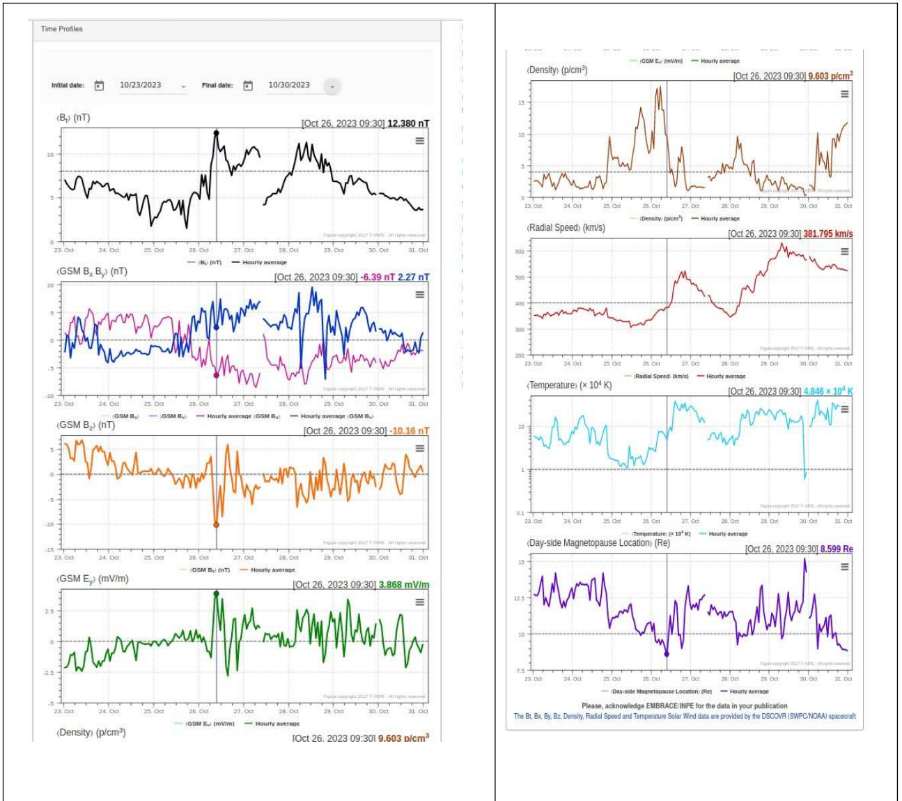
Figure 1 - illustrates a set of parameters observed in the solar wind by the DSCOVR satellite. The measured solar wind parameters can be identified in the following order starting in column 1: Interplanetary magnetic field modulus (IMF), the Bx and By components, Bz component, convection electric field Ey, solar wind density, speed, temperature and the last graph represents the position of the subsolar magnetopause. Note that some profile are repeated in column 2.
